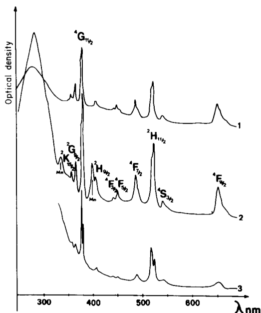
FIG. 1. Absorption spectra of Er 3+ -doped fluoride glasses and Er 3+ -doped ZrO 2 (Y 2 O 3 ). 1—2 wt% ErF 3 : 46 PbF 2 , 22 ZnF 2 , 30 GaF 3 , 2 LaF 3 (mol%), t = 2.2 mm. 2—2 wt% ErF 3 : 46 PbF 2 , 22 MnF 2 , 30 GaF 3 , 2 LaF 3 (mol%), t = 2.6 mm. 3—0.55 wt% Er 2 O 3 : 67 ZrO 2 , 33 Y 2 O 3 (mol%), t = 2.95 mm.
